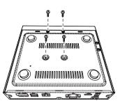
**4.** Re-install the cover of the NVR and fasten screws.
