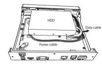
**3.** Place the HDD on the bottom of the device and then fasten the screws on the bottom to fix the HDD.
